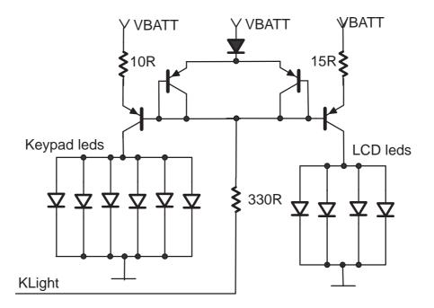
LEDs are controlled by the UEM PWM outputs. Both LEDs are controlled by *KLight* output of the UEM. Current flow through the LEDS is set by biasing the transistor and limiting the current by resistors. Current is set separately to keyboard and LCD leds.
